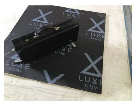
Figure 1: Tapping machine on sample in position 1
